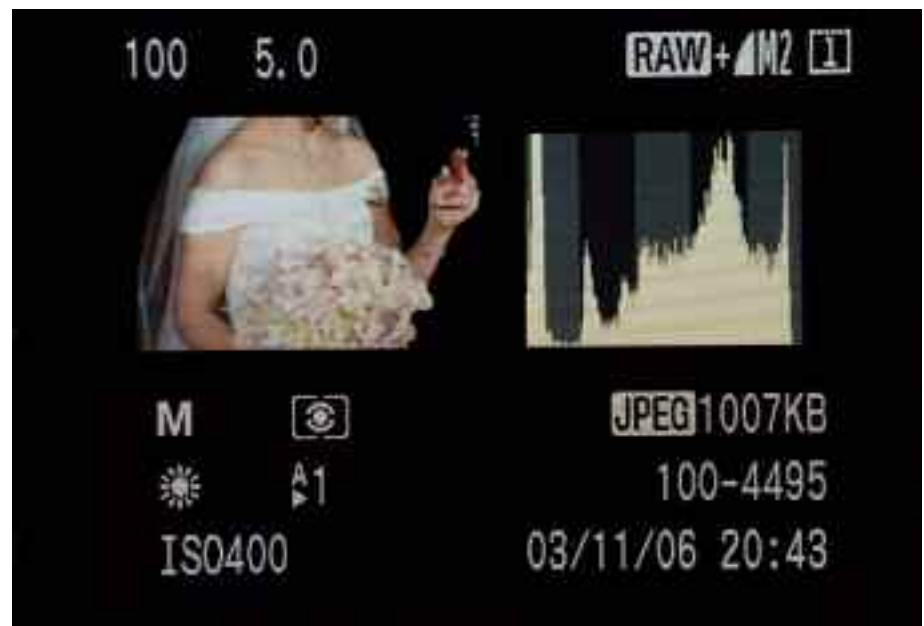
PLATE 5-3. A spike at the right-hand edge of the histogram indicates the image is overexposed.
