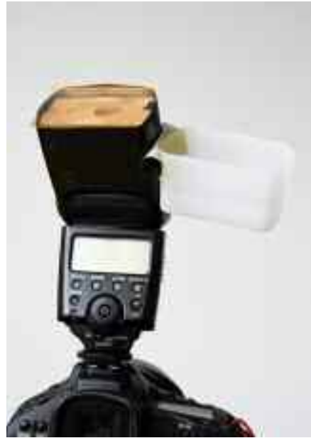
PLATE 9-12 (LEFT). On one of my Stofens, I cut a hole in the top so that the majority of the light can be thrown wherever I want it to go.
